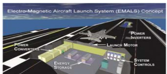
Other advantages includes lower system weight, cost, and maintenance; the ability to launch both heavier and lighter aircraft than conventional systems; and lower requirements for fresh water, reducing the need for energy-intensive desalination. The EMALS uses a linear induction motor (LIM), which uses electric currents to generate magnetic fields that propel a carriage down a
